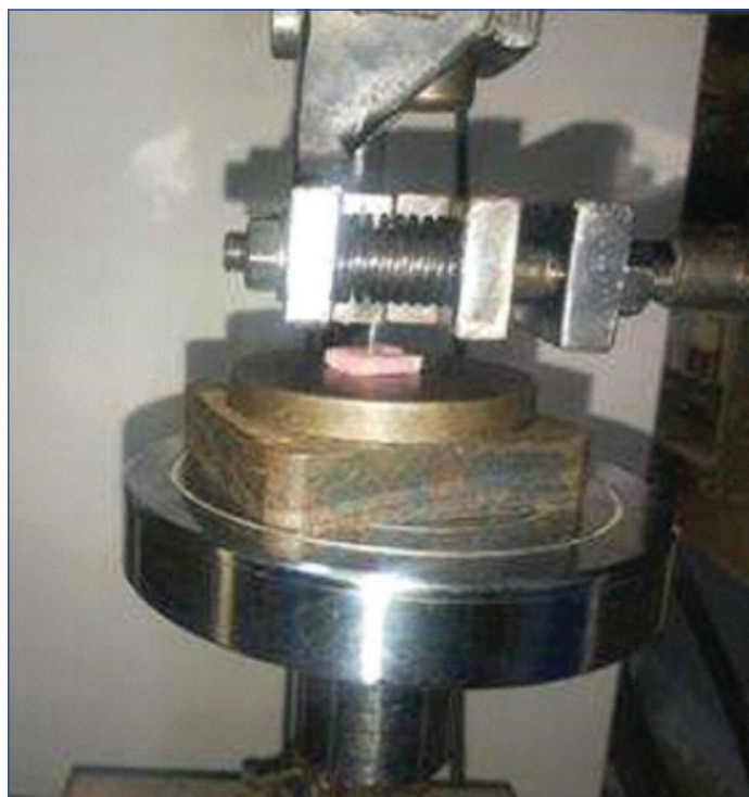
[Table/Fig-2]: Specimen was attached to a support jig and placed on the base of the Universal Testing Machine (UTM).
